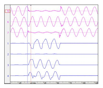
The resulting file is shown above. Here the files were alligned by the position of each data bar. This method is useful for files produced by recording devices that are not GPS synchronized.
