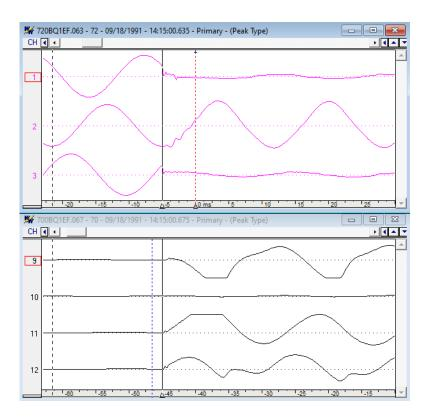
To merge files manually the data bar in each file should first be set to the beginning of the fault as shown above.
